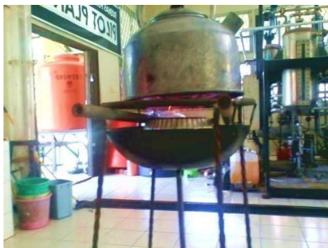
Figure 7: Trial of Boiling Water Using a Waste Cooking Oil Stove
