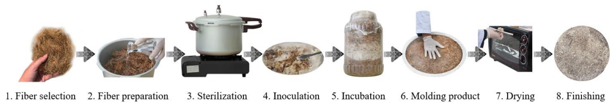
Figure 2: Stages of Making EFB and Mycelium Biocomposite
