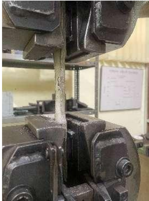
Figure 6. GFRP tensile specimen mounted in the universal testing machine.
