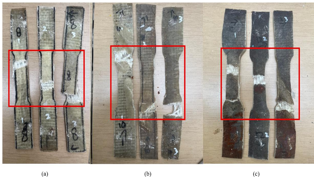
Figure 7. Fractured GFRP tensile specimens after testing, with the fracture zone highlighted: (a) 8 layer, (b) 10 layer, and (c) 12 layer specimen.
