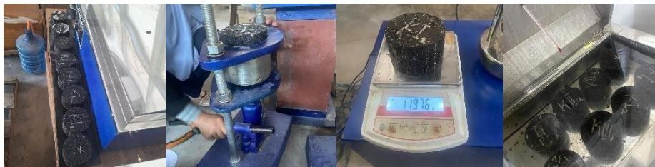
Figure 2. Marshall test specimens of the AC-WC mixture with ESP variations.
