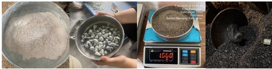
Figure 1. Constituent materials of the AC-WC mixture consisting of eggshell powder, coarse aggregate, fine aggregate, and 60/70 penetration asphalt.
