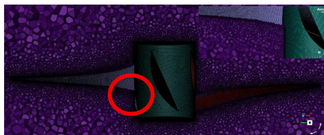
Figure 4. Propeller Volume Mesh
