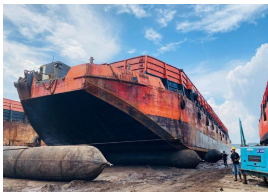
Figure 1. Marine airbag-assisted docking operation of BG. Liana
