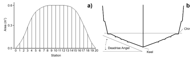
Figure 1. (a) Deadrise Angle, (b) Cross-Sectional Area (CSA).
