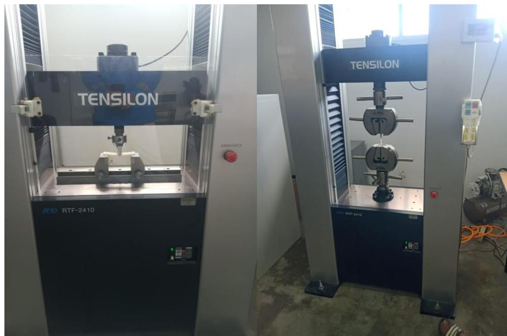
**Figure 1.** Tensile and Bending test processes
