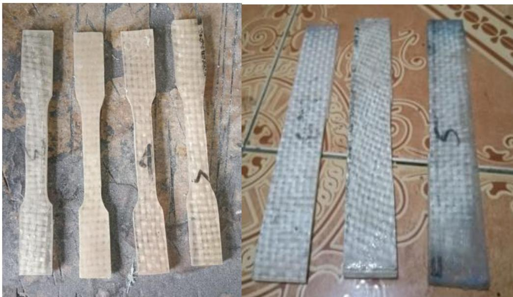
**Figure 3.** Production results of the composite material into specimen shapes ASTM D638-14 dan D790.
