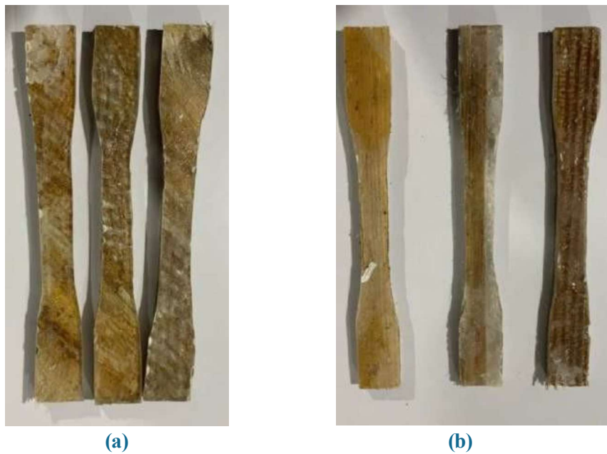
Figure 4. a) 45° fiber direction tensile test specimen; b) 90° fiber direction tensile test specimen
