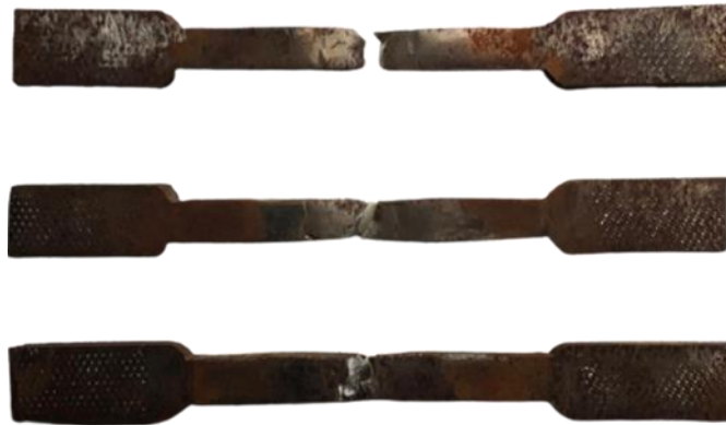
Figure 7. Tensile Test Results of current variation (A) (70, 100, 115 A), current variation (B) (70, 120, 130 A), and current variation (C) (70, 125, 130 A).
